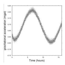
A drift curve measured with a LaCoste "zero-length" spring instrument in the USF lab. The drift is dominated by tidal effects. Measurements are at 1 s intervals. Note the random measurement error due to ground motion in the lab is about 0.05 mGal.
