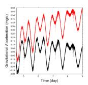
A continuous record of gravitational acceleration in the USF lab, gathered at 1s intervals for several days. The actual drift curve is shown in red, the detrended drift curve s shown in black. The drift curve (red) can be thought of as consisting of two components. The Earth tide varies predominantly on approximately 12 and 24 hr cycles. The tide develops longer period variation (a beat) due to the elliptical motion of the Sun and Moon
