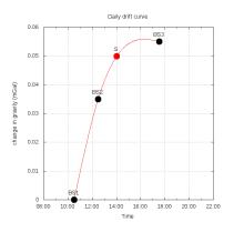
This cubic spline fit was graphed using gnuplot. Gnuplot has great functionality for fitting drift data using a variety of methods. The drift at time S was also determined using Gnuplot. Example codes for estimating the nonlinear drift are provided in the supplementary material.
