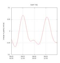
The plot shows calculated upward acceleration due to the Earth tide. In order to correct for the tide the calculated values are added to the the observed gravity.
