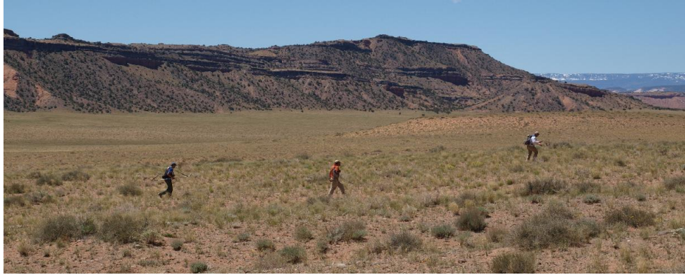
Figure 1: Collecting magnetic data in the San Rafael area. Note that the area is characterized by relatively flat grass covered spaces devoid of outcrops. There are erosion resistant sills capping the sandstone cliffs in the background. Two volcano conduits are in the survey area (not shown on the photo).
